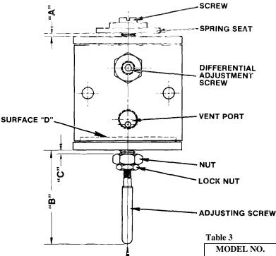
"D" as explained in the Housing Assembly and Stem Maintenance section. Reassemble spring seat (detail 9), adjusting screw, and nut on appropriate end of stem using figure 3 as a guide. Reset dimensions "A," "B," and "C" and reassemble as explained in the Housing Assembly and Stem Maintenance instructions. Recalibrate sensor when assembled.
